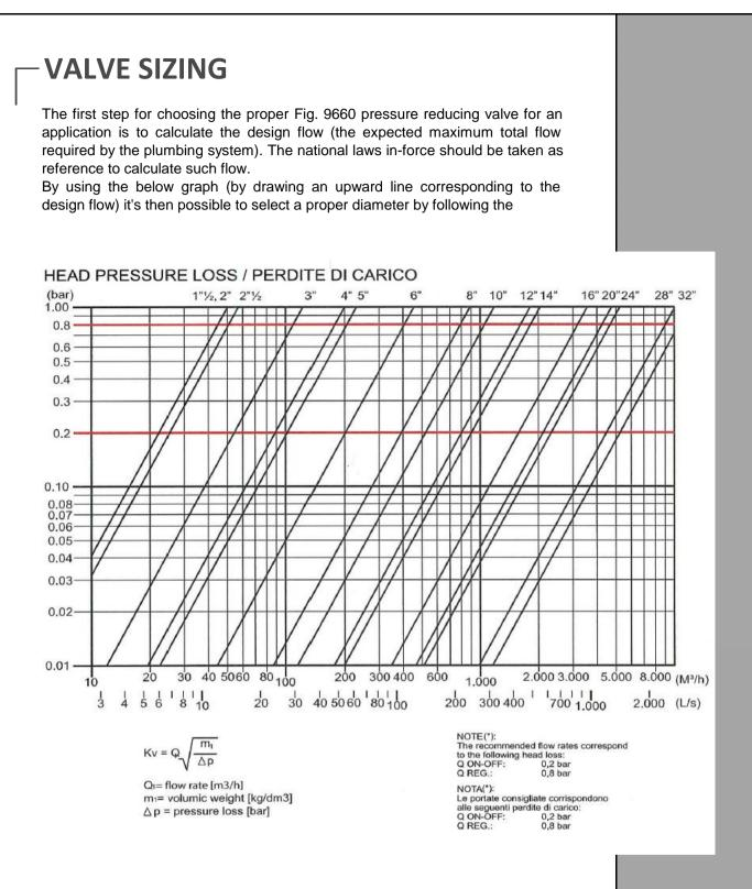
The Fig. 9660 pressure reducing valves have a Max pressure reduction ratio of 3:1, meaning they can reduce the inlet pressure up to 3 times without generating cavitation.
