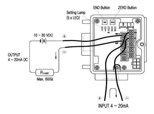
Actuator connection diagram with limit switch.
