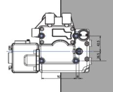
The positioner operates on the force-balance principle by comparing standard signal transmitted from a controller device with the angular rotation on the stem which conveys a positioning amplified pressure
